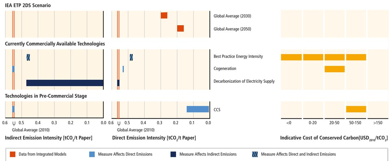
**Figure 10.10** | Indicative global indirect (left) and direct (right) CO<sub>2</sub> emission intensities and levelized cost of conserved carbon in paper production for various production practices/technologies and in IEA ETP 2DS scenario (for data and methodology, see Annex III).
